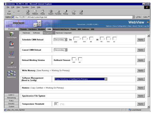
If you have dual redundant CMMs select Copy Working -> Certified & Synchronized with Secondary in the Software Management box as shown below:
