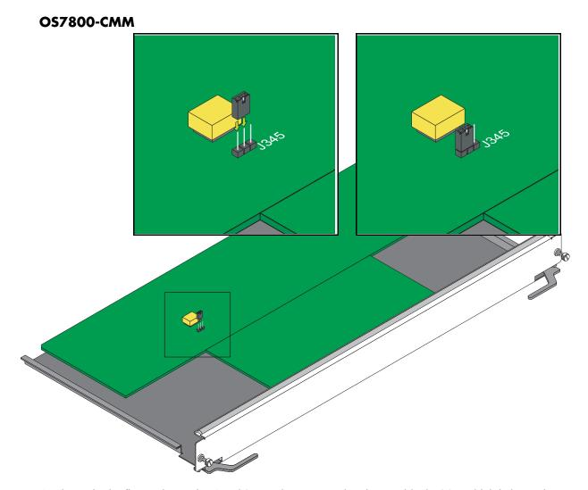
As shown in the figure above pins 1 and 2 must be connected on jumper block J345, which is located near the lithium battery, to ensure a successful FPGA upgrade. (Please note that pin 1 is located the closest to the top edge of the CMM, pin 2 is in the middle, and pin 3 is located facing the bottom edge of the CMM.) If pins 1 and 2 are not connected as shown in the figure above then perform the steps described in "Program Enable Jumpers Not Installed" on page 38 to perform an FPGA upgrade.
