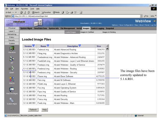
In addition, you should also select **System > System Mgmt > Images > Images in Certified** and **System > System Mgmt > Images > Images in Working** to verify that Certified and Working directories have been correctly upgraded to Release 5.1.6.R01.
