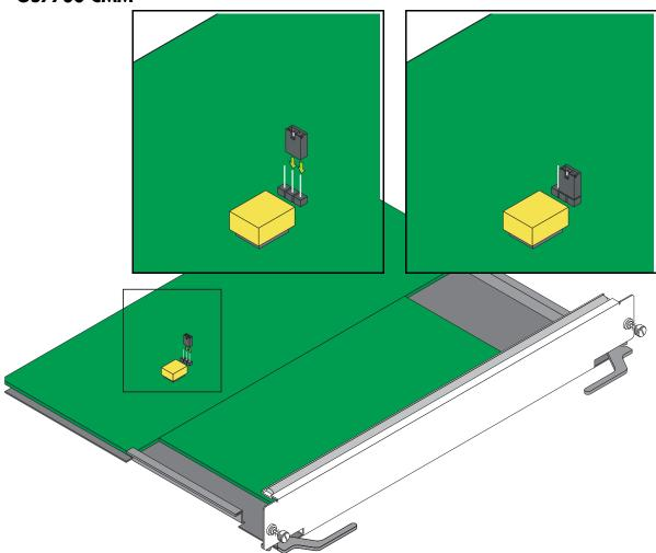
As shown in the figure above pins 1 and 2 must be connected on jumper block J31, which is located near the lithium battery, to ensure a successful FPGA upgrade. (Please note that pin 1 is located the closest to the front panel, pin 2 is in the middle, and pin 3 is located closest to the backplane connector.) If pins 1 and 2 are not connected as shown in the figure above then perform the steps described in "Program Enable Jumpers Not Installed" on page 38 to perform an FPGA upgrade.
